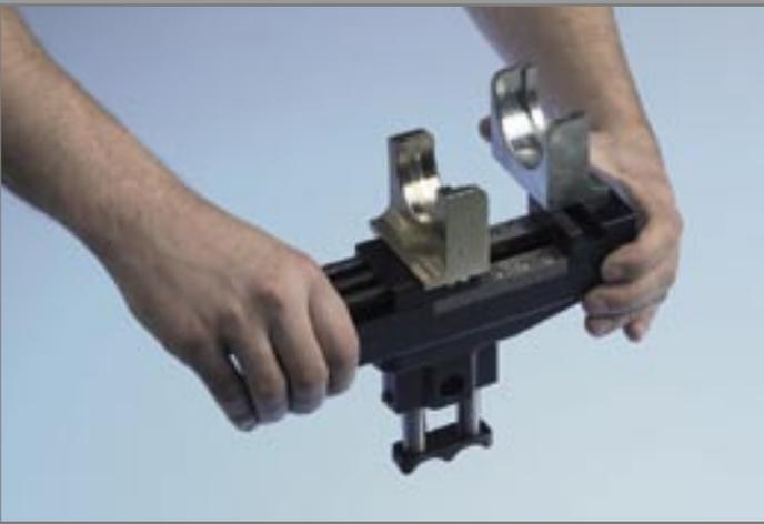
Adaptors for expansion and pressing are available for most standard pressing tools.
