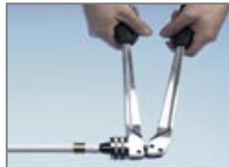
Expansion of the pipe end using the expansion pliers
